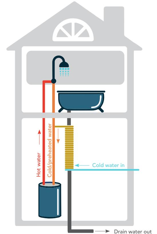
The typical non-storage system usually has a copper heat exchanger that replaces a vertical section of a main waste drain. As hot water flows down the drain, incoming cold water flows through a spiral copper tube wrapped tightly around the copper section of the waste drain. This heat energy transfer preheats the incoming cold water that goes to the water heater or a fixture, such as a shower.
